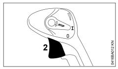
► Press the throttle trigger (2)
