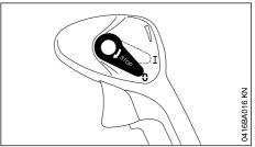
Move the setting (1) to 0. The engine stops and the setting lever springs back to the on position
