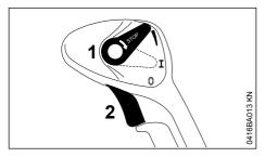
Infinitely variable throttle setting – throttle trigger can be locked in any required position: Move setting lever (1) upwards until required engine speed is reached. To disengage, move the setting lever back to the normal run position I.
