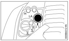
► Press the manual fuel pump at least 8 times, even if the bulb is already filled with fuel
