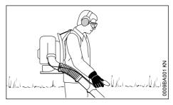
The machine is carried as a backpack. Hold and control the blower tube with your right hand on the control handle.
