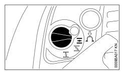
► Choke knob automatically returns to the run position  $\overline{\pm}$  when the throttle trigger is pressed
