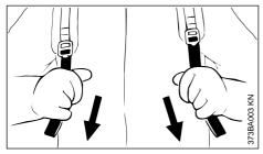
Pull the straps downwards to tighten the harness
